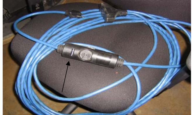
Figure 5 Extension Cord with “built in” Ground Fault Circuit Interrupter
